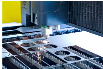
激光切割 / Laser cutting
